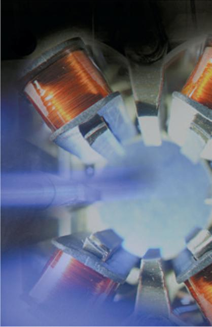
Trietex® uses in its curtain track motors a different drive technology than most other manufacturers. They are synchronous motors that work directly with 110 V / 230 V voltage.
